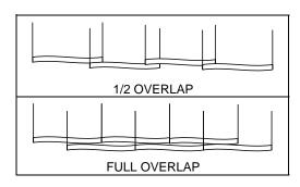
Offers two basic overlap methods. With holes on 1" centers, most any overlap is possible.
